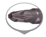
ACR\* stands for Anti-Camout Recess. The ribs on the bit tip engage the fastener recess to reduce stripping, provide increased torque, enhance off-angle drivability, and offer a stick fit that makes screw driving easier.
