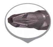
ACR\* stands for Anti-Camout Recess. The ribs on the bit tip engage the fastener recess to reduce stripping, provide increased torque, enhance off-angle drivability, and offer a stick fit that makes screw driving easier.
