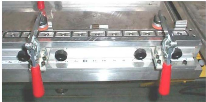
High production mechanical fixture utilizing vacuum and mechanical clamps
