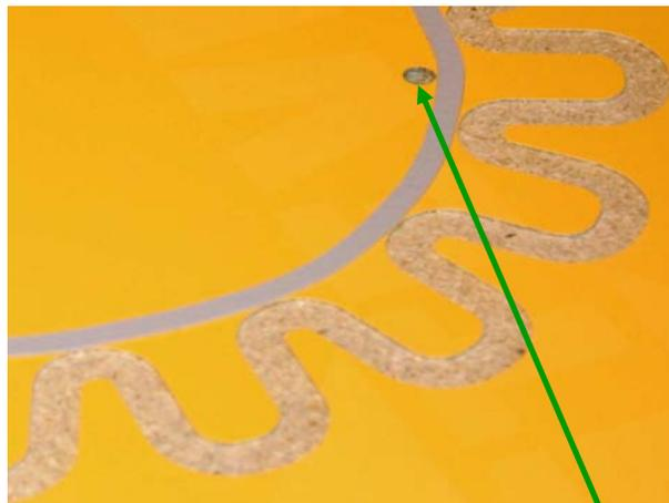
Hole through fixture base for vacuum
