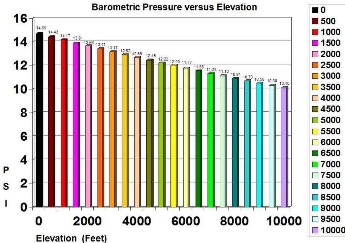
A manufacturing facility located near sea level may experience atmospheric/barometric pressure of approximately 14.7 pounds per square inch (psi) or 1 bar, while a facility located in the Rocky Mountain region may only experience a pressure of 10.1 psi or .68 bar. A value of zero bar would be equal to outer space. Why is this important?
