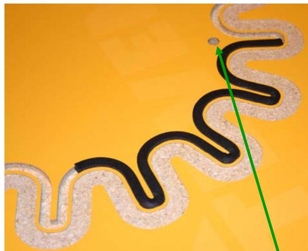
Hole through fixture base for vacuum
